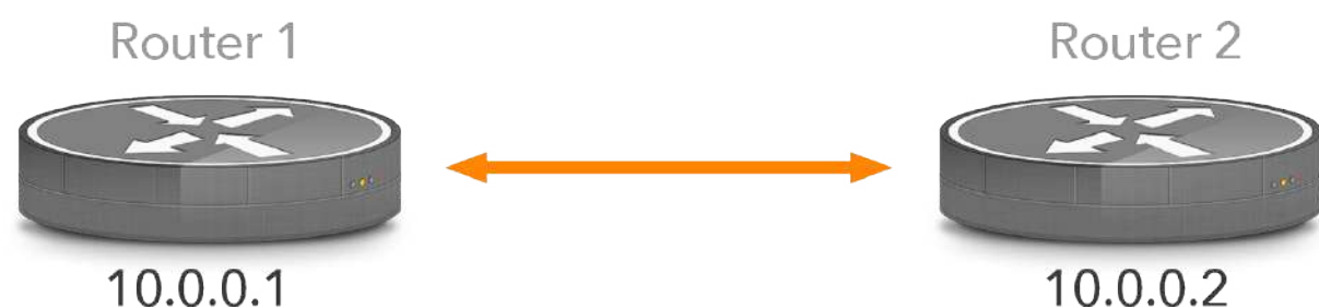
Figure 1: an iBGP session using interface addresses in a small network
